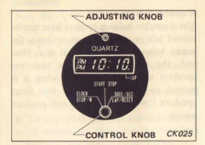
The time is displayed when the ignition switch is in the "ACC" or "ON" position. The clock continues operation even when the switch is set in "OFF" or "LOCK", though the time is not displayed. This digital clock is able to display the time in hours and minutes, or the day (month and date), or it can display minutes and seconds by controlling the control knob, thus being used as a stop watch.
