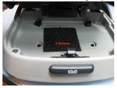
2. Gently pull at console, there should be 2 retaining clips holding the console to the headliner. Unplug main wiring harness from overhead assembly
