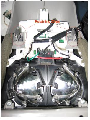
3. Remove the 7 Torx screws. Store in a safe place for installation.
