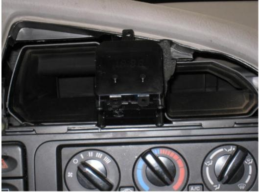
7. Remove the connector from clock by pushing the small tab at bottom of connector
