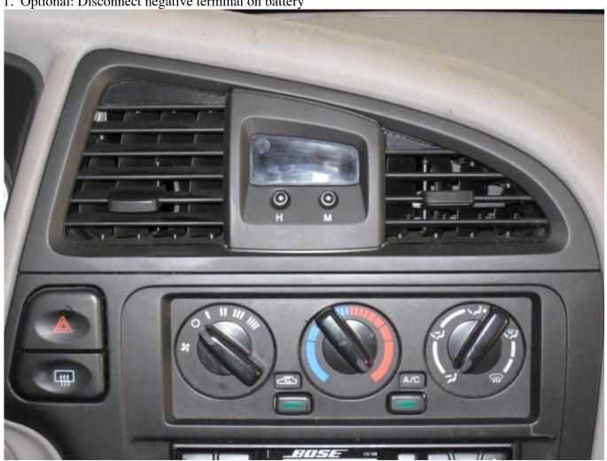
2. Use a flat bladed tool to remove panel. A butter knife works well, but cover with masking tape to prevent damage to trim panel
