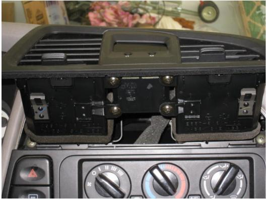
5. Separate the vent panel from the clock by pushing is away from the front of vent panel6. Clock is now separated from vent panel. Put vent panel in safe place
