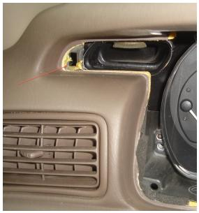
The retaining clips are located here:
