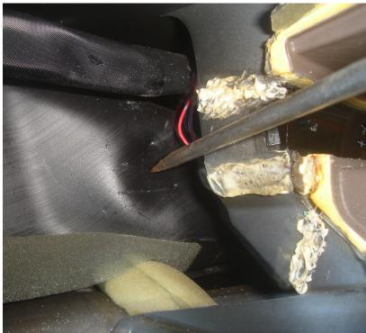
6. Lastly unhook the clock from the wiring harness. A small pait of needle nose pliers comes in handy at this point. It can be a bit fiddly so just keep at it, working form the inside and outside of the locking tab,
