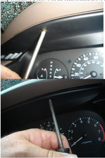
2. Gently insert flat head screwdriver on left (or right) side of bezel by vents and work the bezel out. Gently work on both sides back and forth as well as top of bezel (where screws were removed) until bezel pops off.
