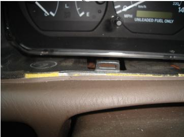
3. There are 4 screws holding the cluster in place, remove all 4 screws. Pull out the cluster and move it towards the driver side. I have found that you do not need to unhook the cluster but it may help if you find
