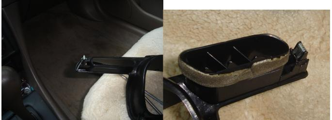
There are also tabs along the bezel that hold the bezel in place
