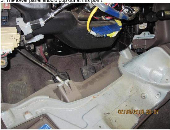
6. Next, remove screws holding lower steering wheel cover in place
