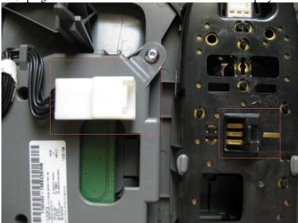
5. Remove the three T10 torx head screws. (If you do not have access to a torx T10 screwdriver you can send the entire assembly in for repair).
