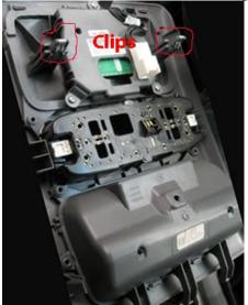
4. Unplug the 2 electrical harnesses connected to the display.
