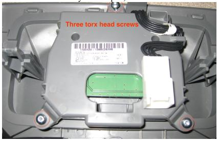
5. Remove the display unit from the console and send off for repair.
