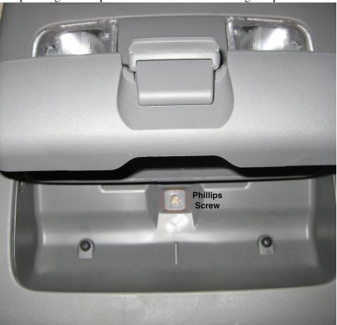
3. With your fingers or by inserting a thin object, pull down on the front of the console. It will require some pressure to release the clips holding the console in place so be patient. There should be 2 metal clips attached to the console, if they are not there, they are probably inside the hole in which the clips reside. Be sure to save and reattach them properly before installation.
