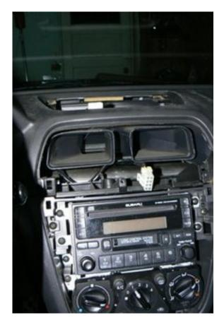
First, I removed the facing around the radio. Then the top piece with the vents and the hazard switch. To do that, I pull out the cup holder and unscrewed the two Phillips screws inside on both sides.
