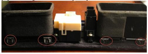
3. Once you have the vent bezel out, remove the electrical plug from the clock.
