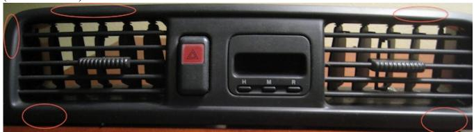
2. Pull the bottom out as it clears, and the top of the vent bezel assembly will follow. The clips holding the bezel in place are shown here. They may pop off during removal so keep an eye out for them.
