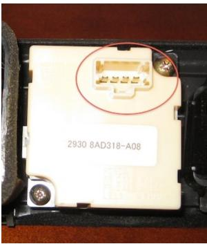
4. Unscrew the two phillips screws that hold the clock in place.
